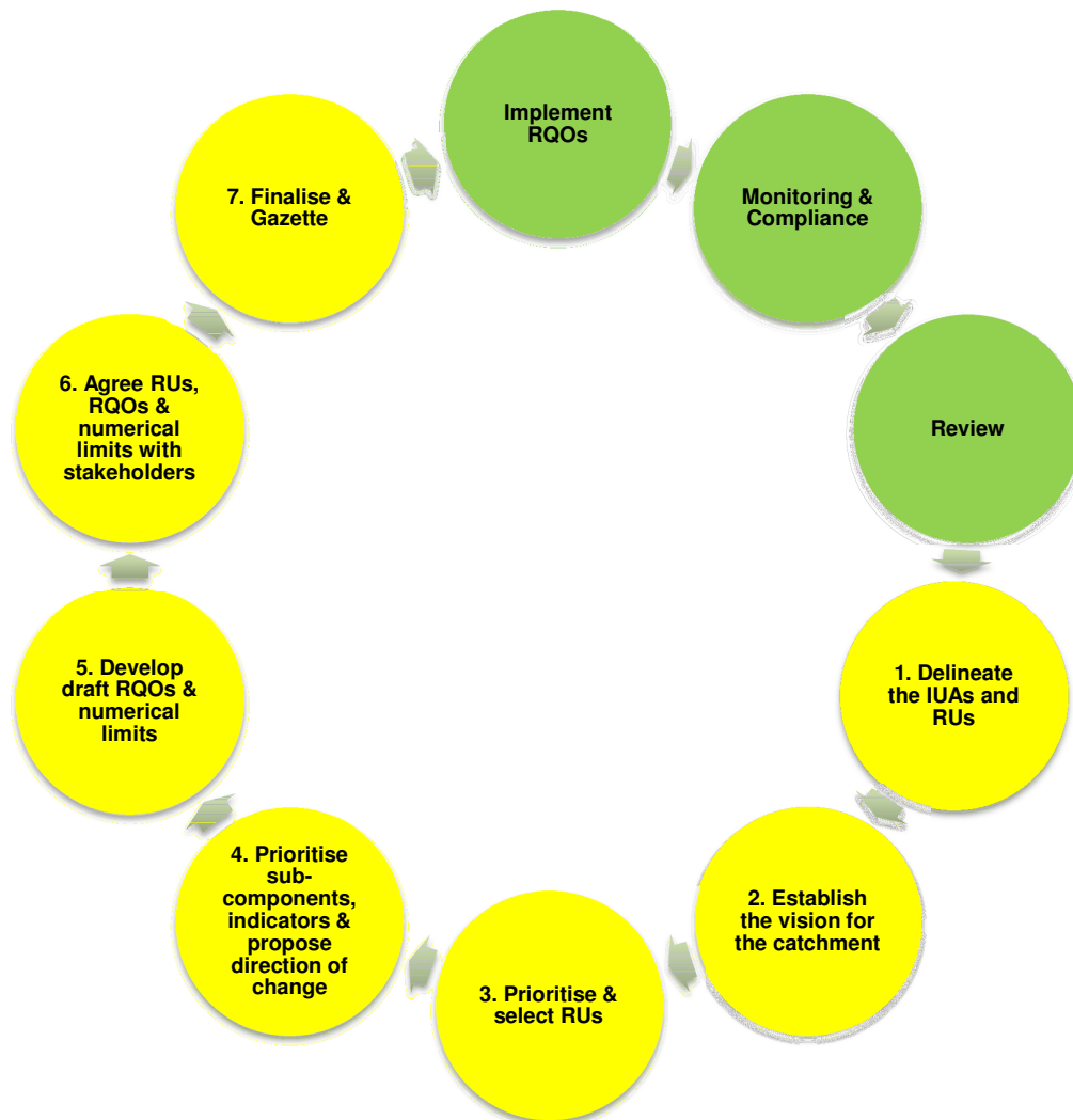
Figure 6. Management of water resources using RQOs; incorporating the seven steps for determination of RQOs and three additional steps to implement the Adaptive Management Cycle.
