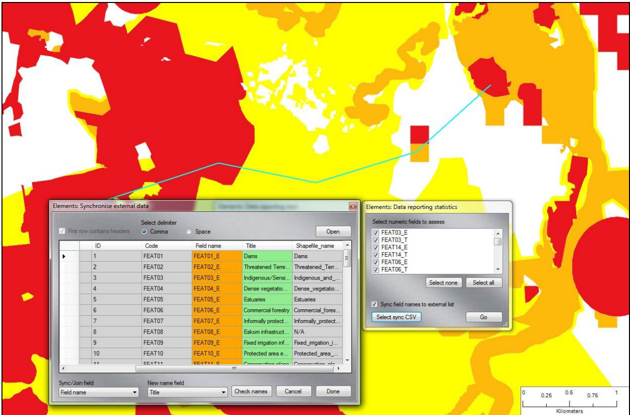
FIGURE 17 THE USER CAN SYNC FIELD NAMES SO COMMON LAYER NAMES SHOW UP ON REPORT
